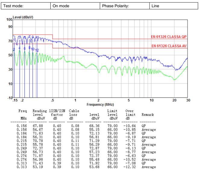
Remarks:level = Reading level + Antenna factor + Cable loss
